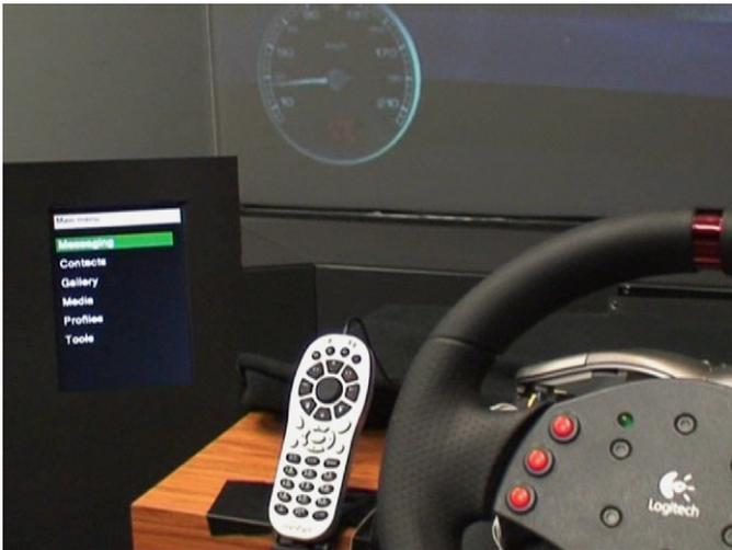
Fig. 1. The visual interaction based on a small screen and phone-like keyboard. The items in the visual menu were displayed in large white fonts and the selected item was highlighted with a green bar.
