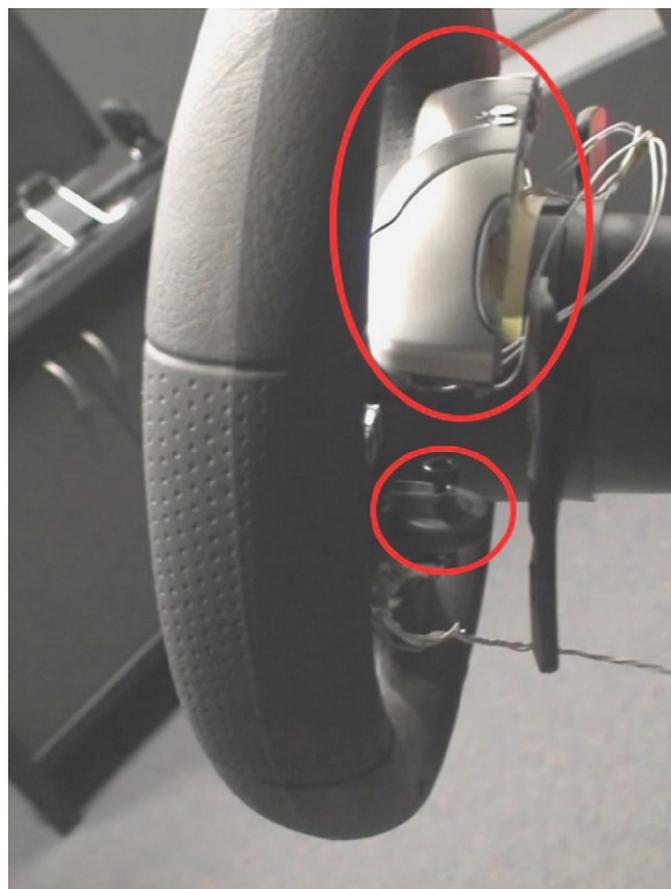
Fig. 5. The interaction device consisted of a scrolling wheel and two mouse buttons. The scrolling wheel enabled the selection of the item in the menu and the two buttons enabled the confirmation (left button) or the cancellation (right button) of the selection.
