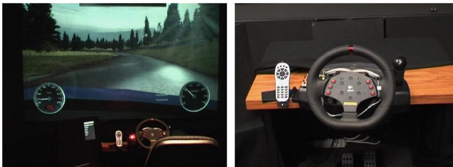
Fig. 3. Car simulator with a large projection screen, steering wheel, and interaction device.
